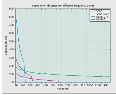
Figure 1. Capacity vs. distance comparison for different wireless systems calculated with the parameters shown in Table 2.
