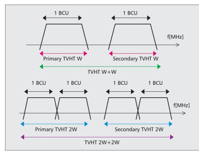
**Figure 3.** *TVHT PHY channel configurations: TVHT W, 2W, W+W, and* 2*W*+2*W*
