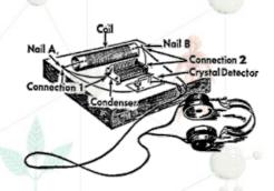
The antenna attaches to the nail that connects with the coil and razor blade (A). The ground wire attaches to the other nail, where the coil connects with the earphones (B). Hook up the headphones,
