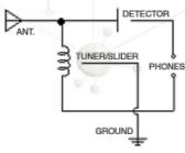
Refer to the schematic for wiring and connections. Wind the coil 100 turns around the tube. #22 AWG wire is recommended, but it is likely that whoever was in the field used whatever gauge was in the scrap coil, motor, or transformer they were cannibalizing. Spray / paint the coil with lacquer (or whatever is handy) to set it firmly. Scrape off whatever paint or varnish may be on the wire used for the
