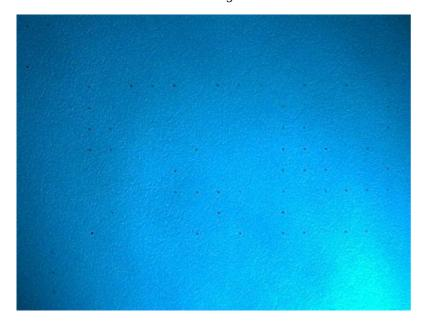
The illumination is from the lower right; to the upper and lower left of the image, the corners of another repetition of the dot grid are visible.
