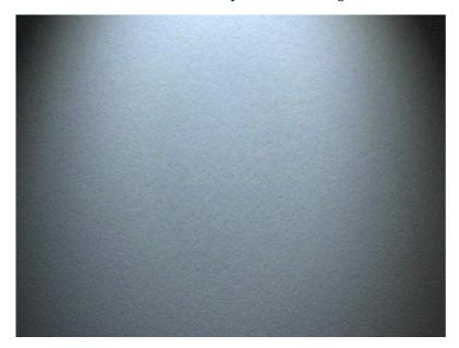
This is an image of a portion of the dot grid under 60x magnification. Now the dots are easy to see, but their overall structure is hard to discern because the microscope field only includes a few dots at a time.
