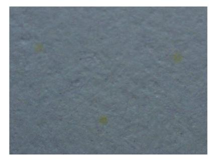
This is an image of one repetition of the dot grid from the same Xerox DocuColor 12 page, magnified 10x and photographed by the QX5 microscope under illumination from a <a href="Photon">Photon</a> blue LED flashlight. Note that the increased contrast under blue light allows us to see the entire dot pattern clearly.
