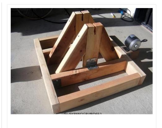
A 12-volt DC motor or higher is recommended. The wattage of the motor depends on what you want to power. The motor should be securely mounted to the stand. Mount the motor at a distance that will tightly secure the drive belt on the motor shaft. The belt and motor shaft should spin concurrently – make sure there is no slipping between them.
