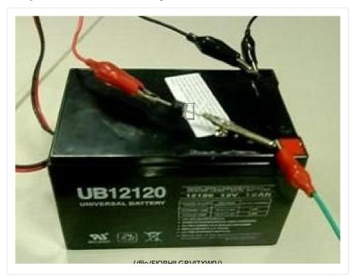
The battery should be connected in series with the motor and diode. The negative lead form the motor should attach to the negative terminal of the battery. The positive lead from the motor should be attached to the diode, and the diode to the positive terminal of the battery.
