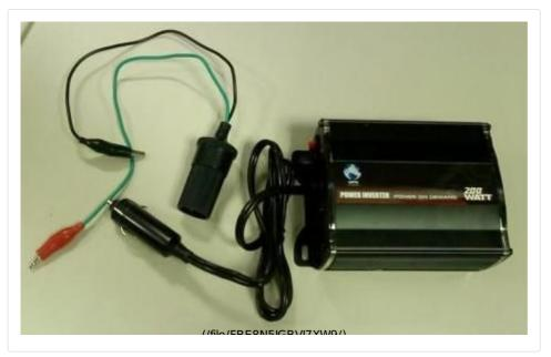
You could use an adapter to connect the battery to the inverter, or you will need to solder or tape the battery's leads to the inverter so the circuit is secure. Be sure to correctly connect the positive and negative terminals of the battery to the inverter or you will blow the fuse in the inverter.
