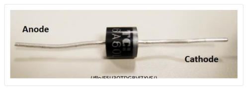
Make sure the diode is only allowing current to flow from the motor to the battery. The cathode should be pointing towards the positive terminal of the battery.
