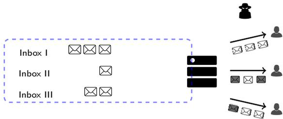
**Figure 3:** Provider stores messages destined for assigned clients in a particular inbox. When users pull messages from the mix node, the provider generates cover messages to guarantee that the adversary cannot learn how many messages are in the users inbox. The messages from the inbox and dummies are indistinguishable.
